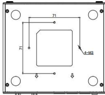
2. After finish installing the internal parts (see below), then install the bottom plate, then install the four M2.5\*6 screws.
